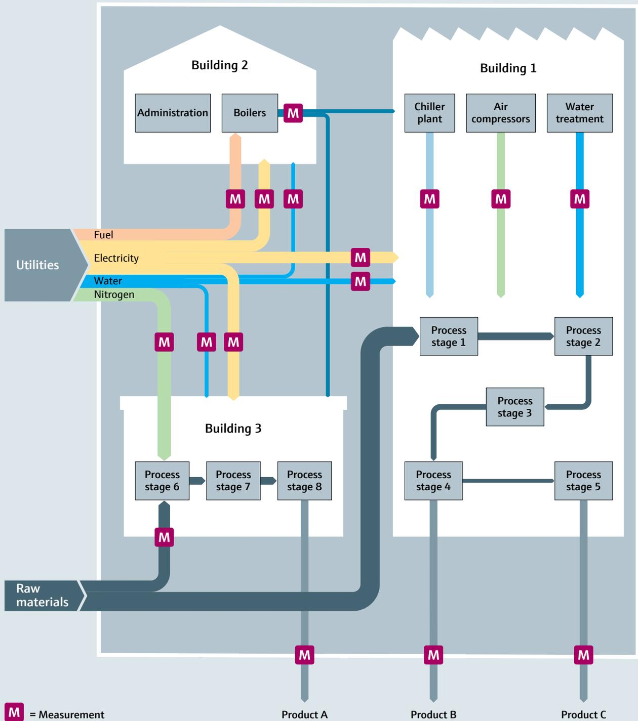
Procedure for measuring material and energy flows as the basis for sustainable energy management
